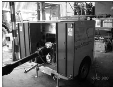
**Fig. 1. Fromet Sigma 5 pto dynamometer**
