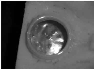
**Fig. 4. The “gel like” B70 blend at -10°C**
