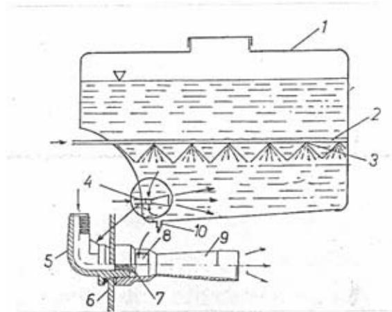
**Fig. 1. Combined stirring system with only one ejector**
