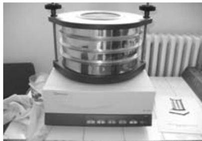
**Fig. 3. Sieving machine AS300**
