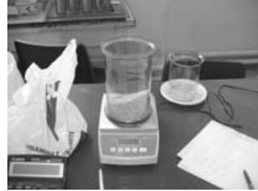
Fig. 6. Weighing one mix sample
