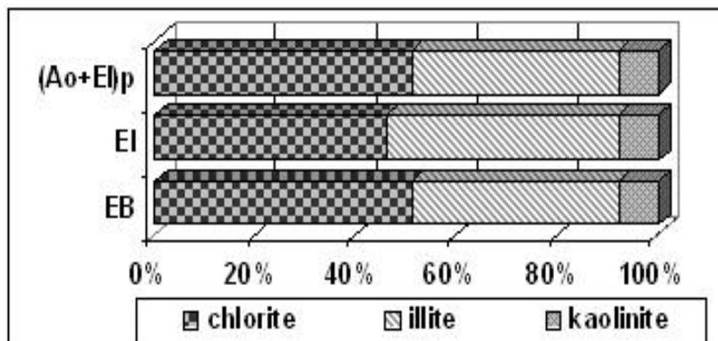
**Fig. 3. The mineralogical composition of the clay (< 2µm)**
