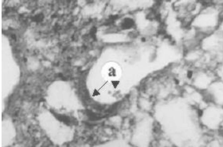
**Fig. 1.** *Impure clay coatings with microorganisms (P2); 75X, N II*
