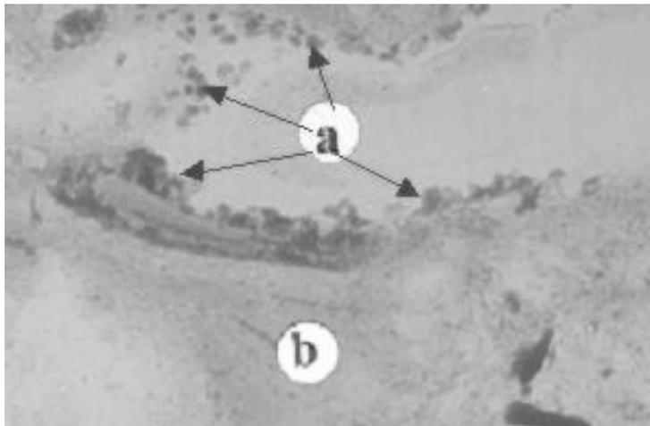
**Fig. 2.** *Impure clay coatings with microorganisms (P1); 184 X, N II*
