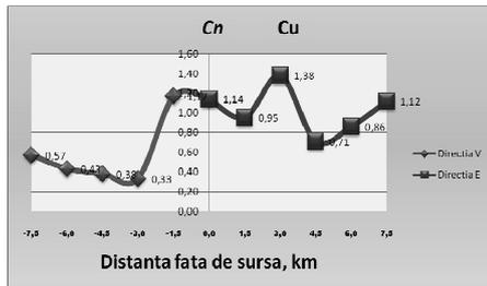
**Fig. 3. Variation of coefficients exceeding the maximum normal values of copper on the NE-SW directions**
