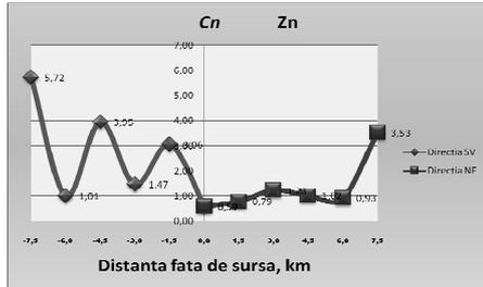
**Fig. 7. Variation of coefficients exceeding the maximum normal values of zinc on the NE-SW directions**
