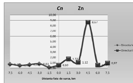
**Fig. 6. Variation of coefficients exceeding the maximum normal values of zinc on the W-E directions**
