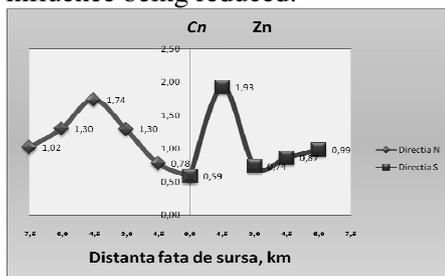
**Fig. 5. Variation of coefficients exceeding the maximum normal values of zinc on the N-S directions**
