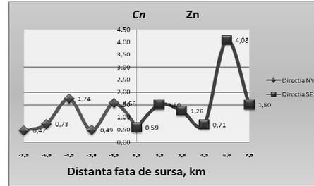
**Fig. 8. Variation of coefficients exceeding the maximum normal values of zinc on the NW-SE directions**
